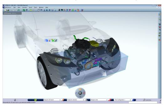
Visual 3D dashboards present the necessary engineering or enterprise information in the context of the 3D design for quicker decision-making. For example, Designers can track the weight of the assemblies using the weight dashboard to identify components with incomplete or missing weight definition.
