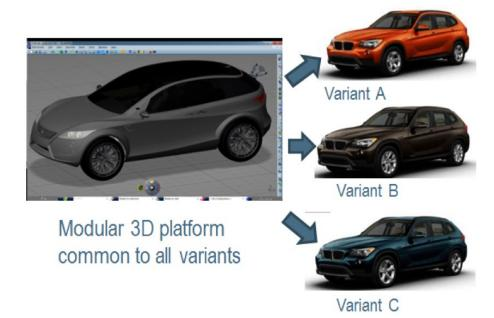
Engineers can turn features "on and off" using dynamic filters in CATIA to access 3D designs instantly to review ad-hoc design configurations. This enables designers to ensure their designs are compatible with all variants, helping support effective design modularization. For example, a designer making a change to the bumper accesses the 3D design for the fog light variant from the modular product structure to check for any issues.
