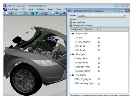
This is only possible since we don't constrain assemblies within files but manage them in a database, enabling us to dynamically pull any components into the design session.
